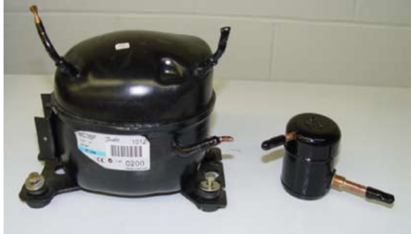
Figure 4 Mini-Compressor alongside Reciprocating Compressor of Equivalent Capacity
