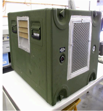
Figure 3. Mobile Satellite Antenna Electronics Case with the Rack Mounted Cooling System inside
