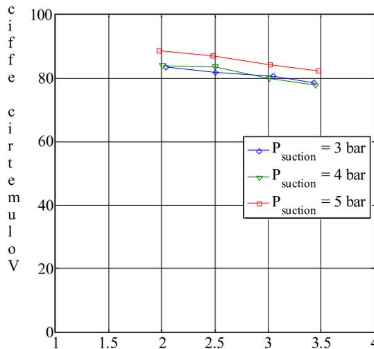
Figure 3 Volumetric Efficiency Vs. Pressure Ratio at 6,000 RPM
