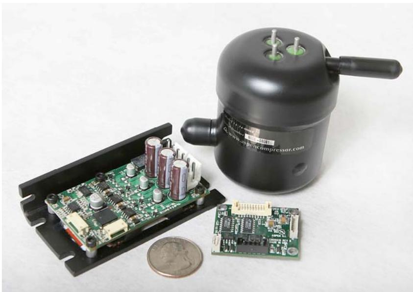
Figure 1. Miniature Refrigeration Compressor shown with Motor Drive, Controller & a Quarter Coin
