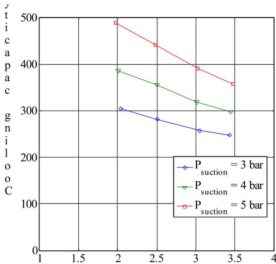
Figure 2 Cooling Capacity Vs. Pressure Ratio at 6,000 RPM
