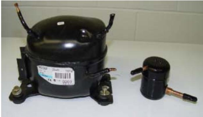
Figure 4. Size Comparison between the New Miniature Compressor (1.4cc displacement) and DC driven Reciprocating Compressor with 20% Less Cooling Capacity
