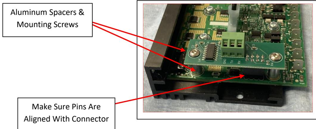
Step 3 – Connect the appropriate communication wires the adapter board. The board will interpret commands sent to the RX connection and provide information on the TX connection.
